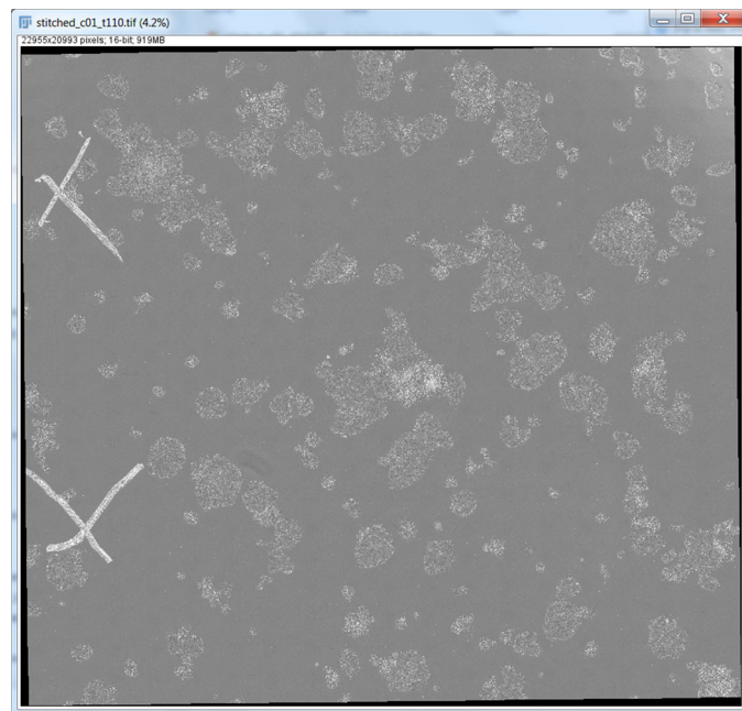
Figure 1. A stitched image with 18 \times 22 tiles and linear blending. The image has 23K \times 21K pixels. It has a 1GB file size.
